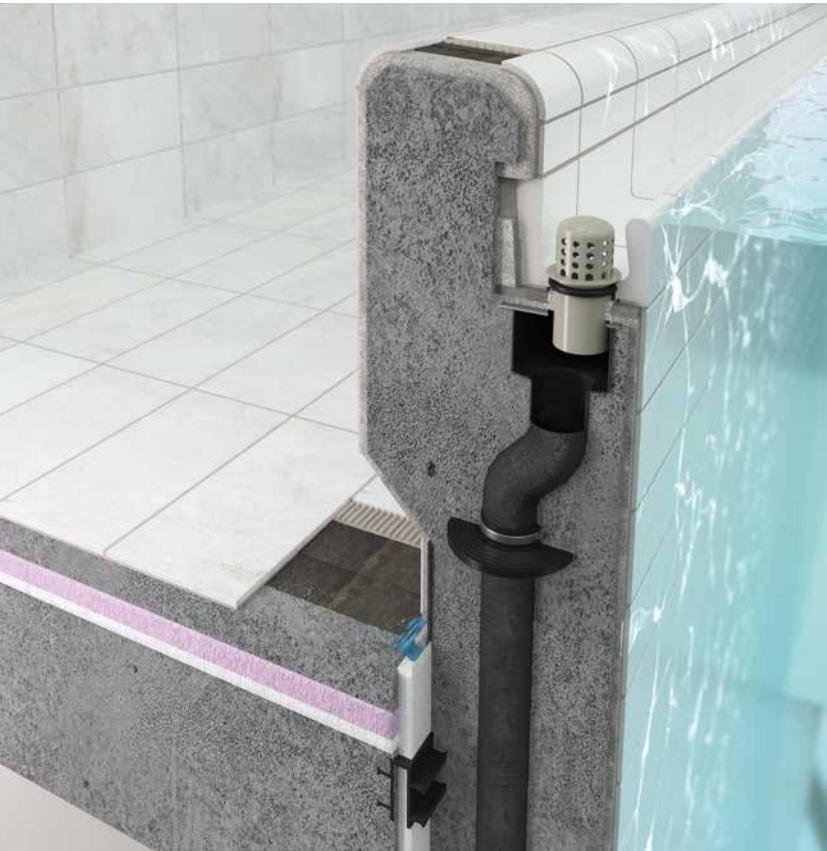
3D-Rendering · 3D rendering Beckenkopfsystem Wiesbaden · Wiesbaden pool edge system Therapiebecken · Therapeutic pool
